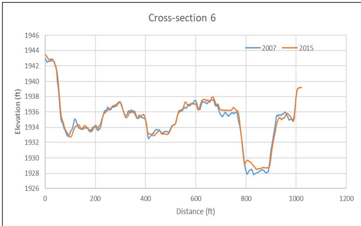
Figure 23. Cross-section 6 elevation data from 2007 and 2015 LiDAR.
