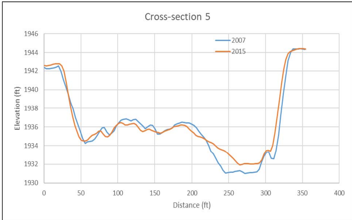
Figure 22. Cross-section 5 elevation data from 2007 and 2015 LiDAR
