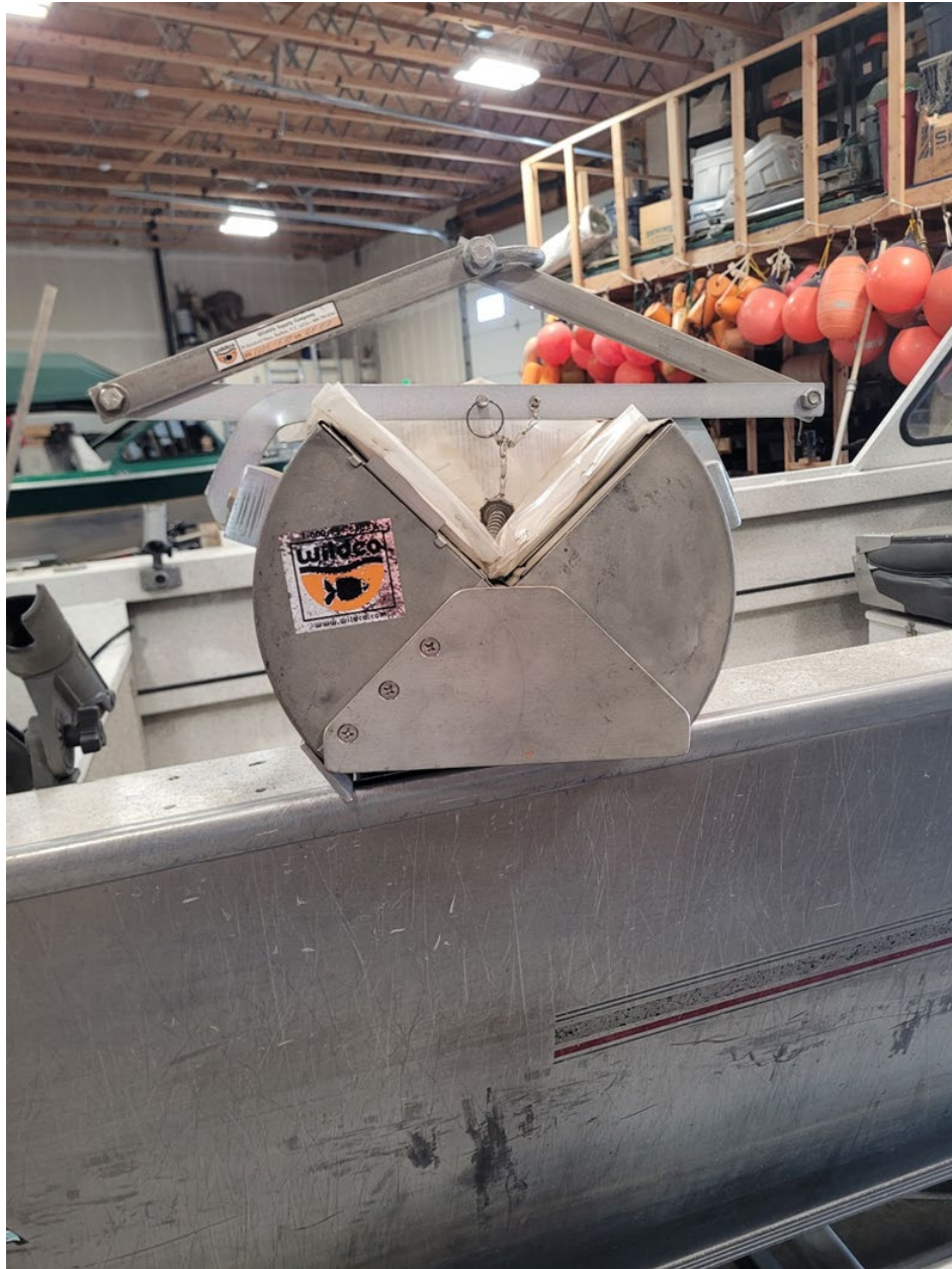
Photo 1. Ponor grab sampler used of sediment sampling in Bonneville Reservoir, Columbia River.
