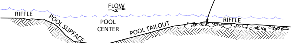
1 12 PROFILE VIEW - TYPICAL POOL AND RIFFLE NOT TO SCALE
