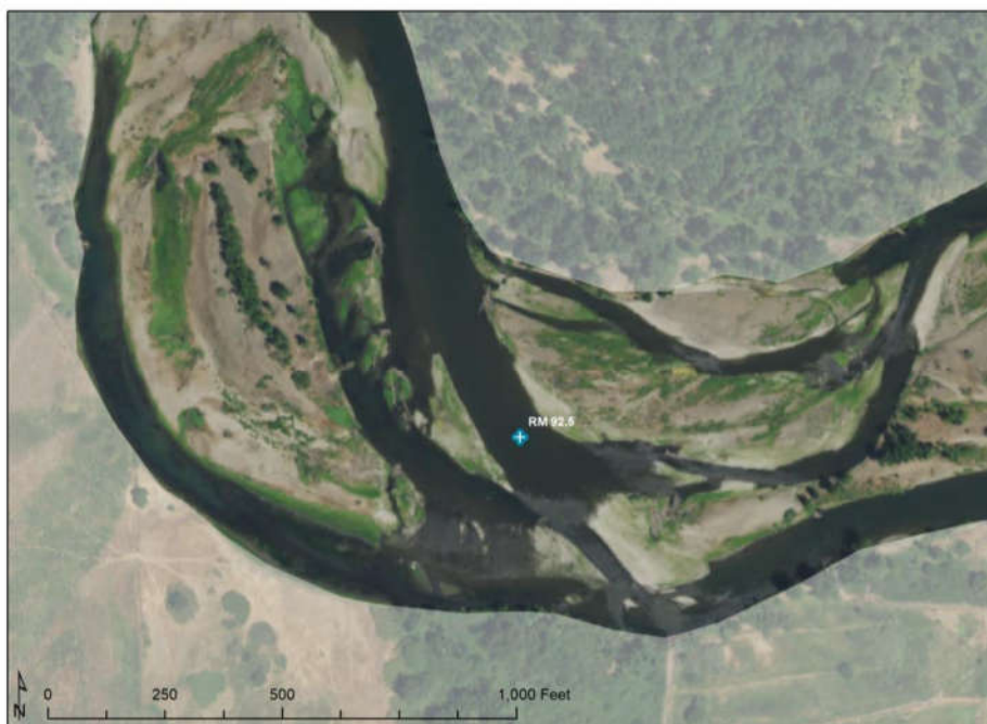
Figure 10. An example of an unstable channel within the Wapato project reach (RM 92.5). The channel morphology indicates that channel migration and bedload transport rates are high throughout the reach and
