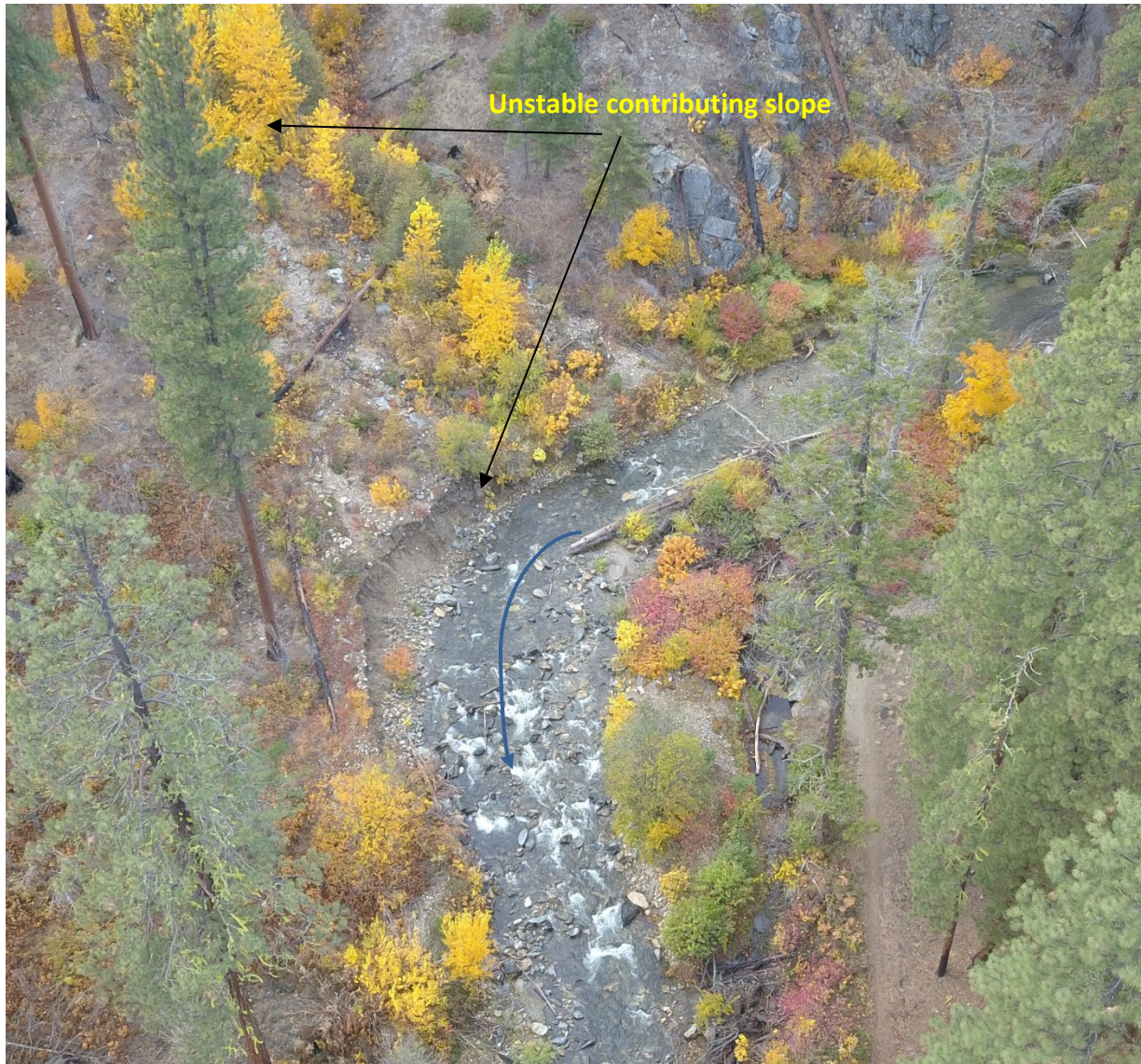
Figure 11. Aerial image (Oct 2021) of river right unstable debris-flow hillslope (RM 4.25) that continues to contribute sediment to the channel.
