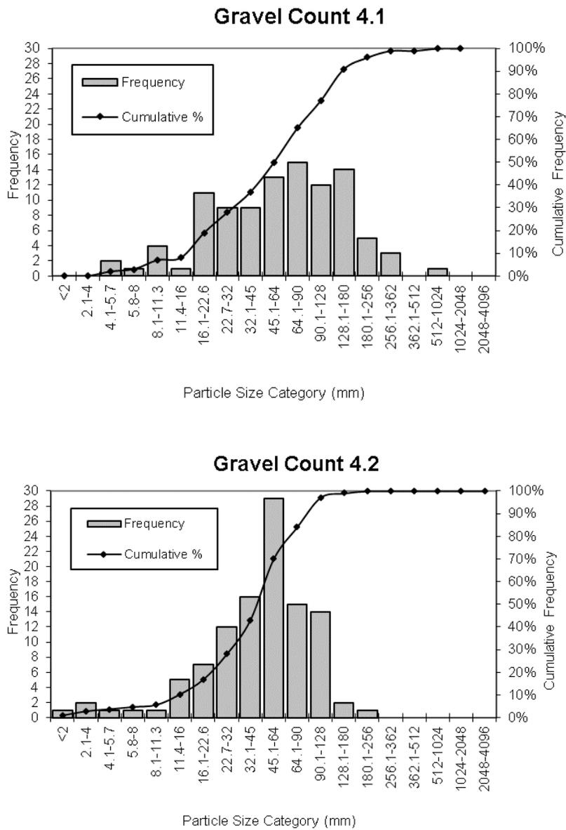
Figure 41. Cumulative grain size distribution for Gravel count 4.1 and Gravel Count 4.2.
