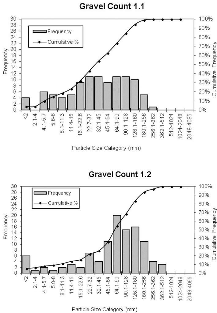
Figure 20. Cumulative grain size distribution for Gravel Count 1.1 and 1.2 (Reach 1).
