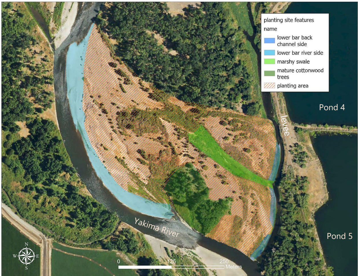
Figure 4. Features of planting site. The lower bar surfaces are inundated by the average winter flow (4,000 cfs) and do not support perennial vegetation. The grove of mature cottonwood trees does not need additional planting, and the marshy swale is too wet for terrestrial plants. The red hashed area is at appropriate elevations and of suitable substrate for riparian plantings. Aerial image is from July 2023.
