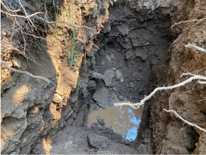
TP-1, groundwater perched on bedrock
