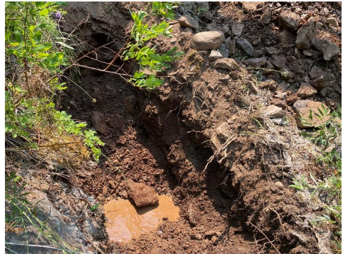
TP-4, groundwater perched on bedrock
