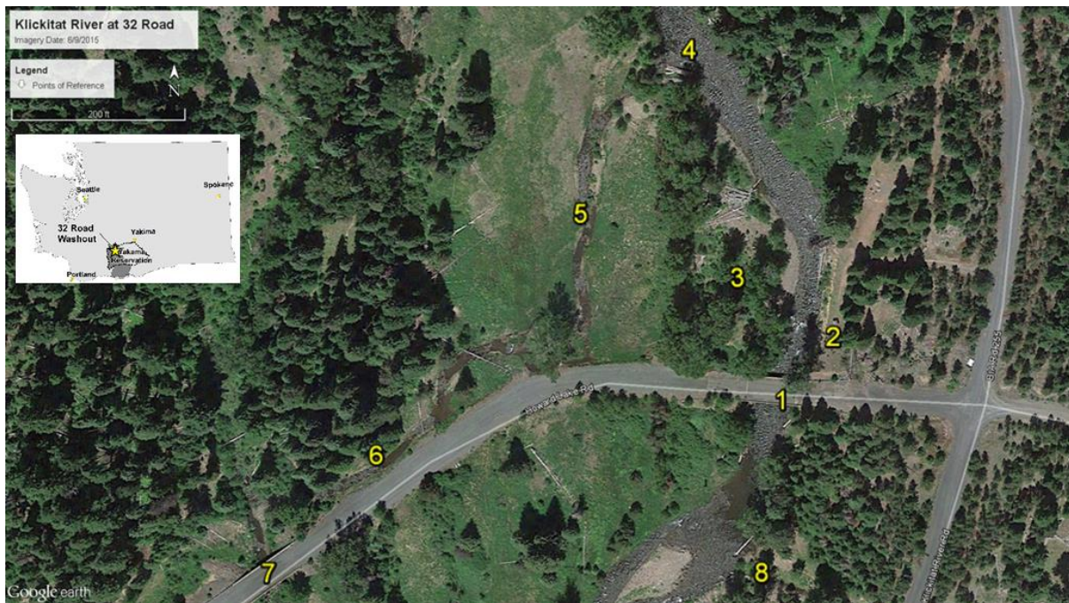
Figure 3: Point 1. East bridge 2. Eroding bank 3. Alluvial deposits 4. Side Channel inlet 5. Side Channel 6. West bridge 7. 32 Rd.
