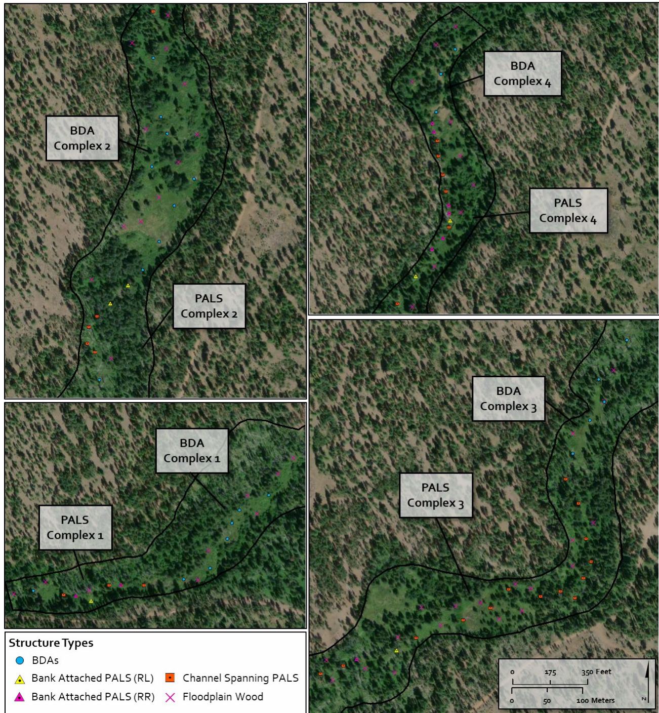
Figure 24. Restoration design outlining structure type and location for complexes on Brush Creek. Structure coordinates can be found below in Table 8.
